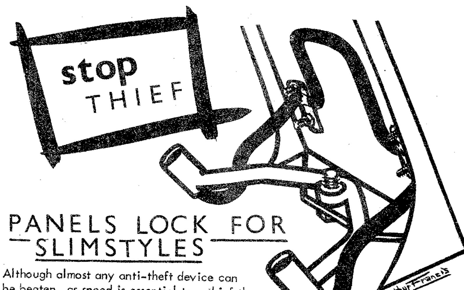
be beaten, as speed is essential to a thief the side panels lock will almost certainly mean that he will move on to another machine where the panels can be off in seconds rather than minutes! With a padlock instead of the bolt this device is even better!
