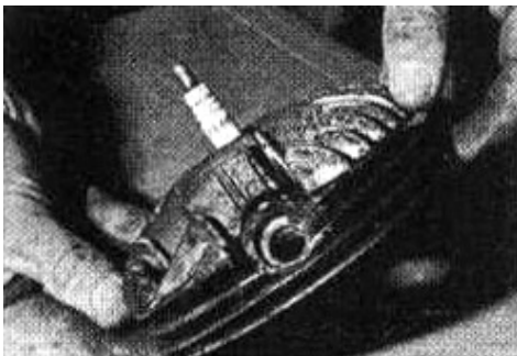
This special head, from a 200cc Lambretta, has a centrally situated sparking plug. Coupled with higher ratio it gives a useful power boost. Other plug can be kept in place as a reserve
