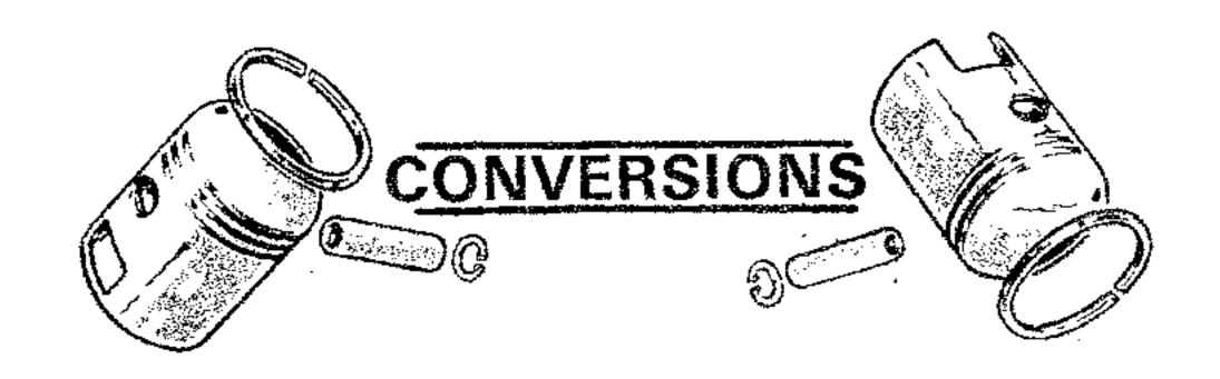
The heart of a conversion is the new piston usually between 3 – 5 mm larger in diameter than the original. The barrel is bored and honed to suit, a new cylinder head, gaskets and carburettor alteration being necessary.
